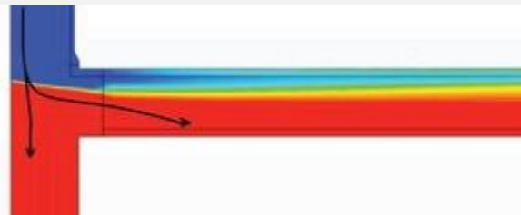
02 – Development of the flow in a tee joint with the addition of a flow rectifier.
